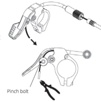
Step 5. Attach the cable end nut to the dropper post by sliding it in to the allocated slot on the dropper post. For internal dropper posts the cable outer simply fits in to the recess (see diagram).
