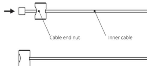
**! Make sure you have orientated the cable end nut correctly, the inner cable end should be flush when installed**
