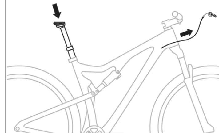
Step 7. Attach the remote lever to the handlebar, position this close enough to the handlebar grip that the rider's thumb can press the lever. Once the lever is attached securely the cable tension must be adjusted. This can be done by using barrel adjuster. The cable should have 1-2mm of play and should not be under tension. If tension is too high the dropper post may actuate unintentionally.
