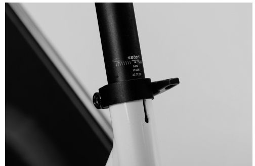
Fig. 14: Marking for the minimum seat post insertion depth
