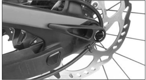
The lever can now be pulled slightly away from the axle and turned into any position you choose. To retighten the axle, reposition the lever on the axle in a comfortable position and tighten the torque again.
