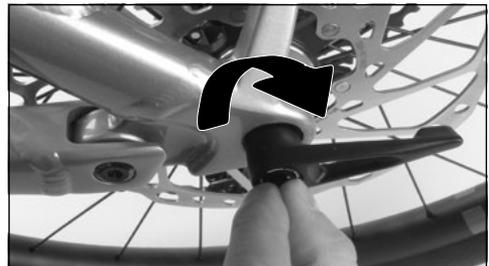
5. To release the axle, turn the lever anticlockwise. If you cannot apply enough force to the lever in the current position, follow steps 1 to 4 in reverse. Then you can adjust the position of the lever to make it easier to loosen.
