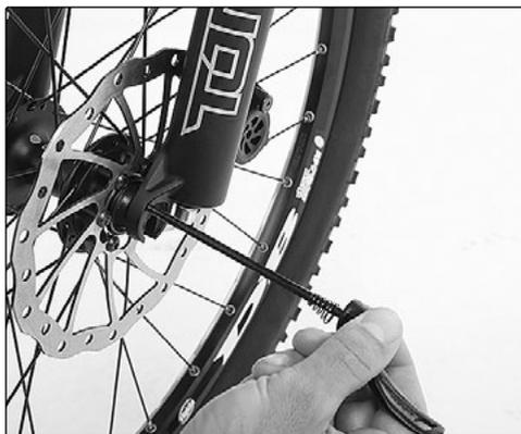
2. Place the springs and the nuts on the bolt. Turn the right end now protruding from the hub and the nut clockwise.
