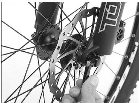
2. Turn the nut counter-clockwise until the wheel can be removed from the frame or front forks without any great effort. Should the nut come right off the screw, please ensure that the little springs do not get lost.
