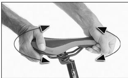
Try to move the saddle in its clamp with alternate up and down movements. It should not be possible to move the saddle.
