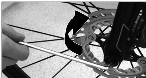
3. Then adjust the torque to the manufacturer-specified value using a torque wrench, but never exceeding 16 Nm.
