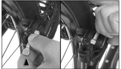
**4. Please ensure that the brake blocks correctly cover the rim shoulder when operated.**
