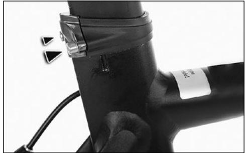
For clamping without a quick release, a hexagon socket and a torque wrench of the appropriate size are required. Please also consult your dealer.
