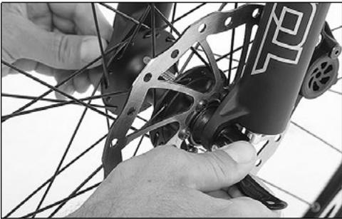
5. Now turn the nut or the Allen key bolt head until the excentric lever, when turned around its bearing more than 90° to meet slight resistance (it now forms an approximately straight line extension of the hub axis).
