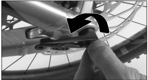
4. Once you have tightened the axle enough, position the lever so that it points towards the front-end of the bike and slide the lever onto the axle. Now turn the fixing screw 180° clockwise to secure the lever against working itself loose.
