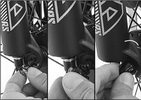
3. On saddle stem quick release levers: instead of the nut, turn the bolt with the Allen key head itself clockwise.
