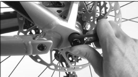
2. Tighten the axle to achieve a secure fit by using the lever and applying manual force. Do not exceed a tightening torque of 16 Nm.
