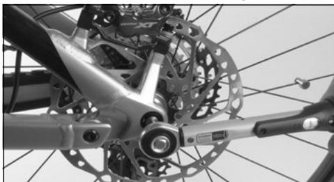
4. To remove the thru axle, it must be unscrewed using an Allen key.
