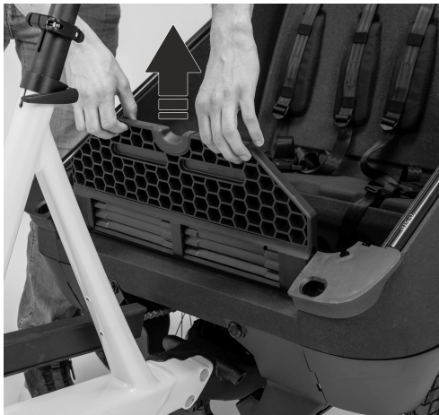
Fig. 21: Pull the footboard upwards
