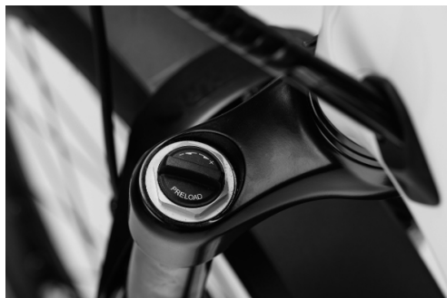
Fig. 17: Suspension fork preload adjuster
