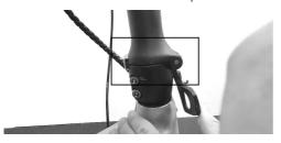
→ Lock the lever on the stem in the upward position.
