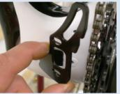
first Loosen the 2.5mm allen wrench screws of the anti-chainsuck-cap and remove the cap
