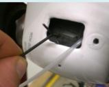
Now you put the cable through the down tube until you can pull it out of the hole at the BB shell.
