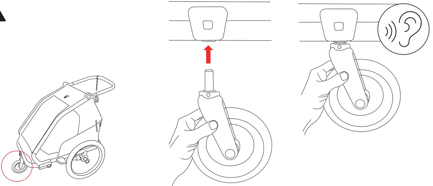
BUGGYRADDEMONTAGE / BUGGYWHEEL DISASSEMBLY
