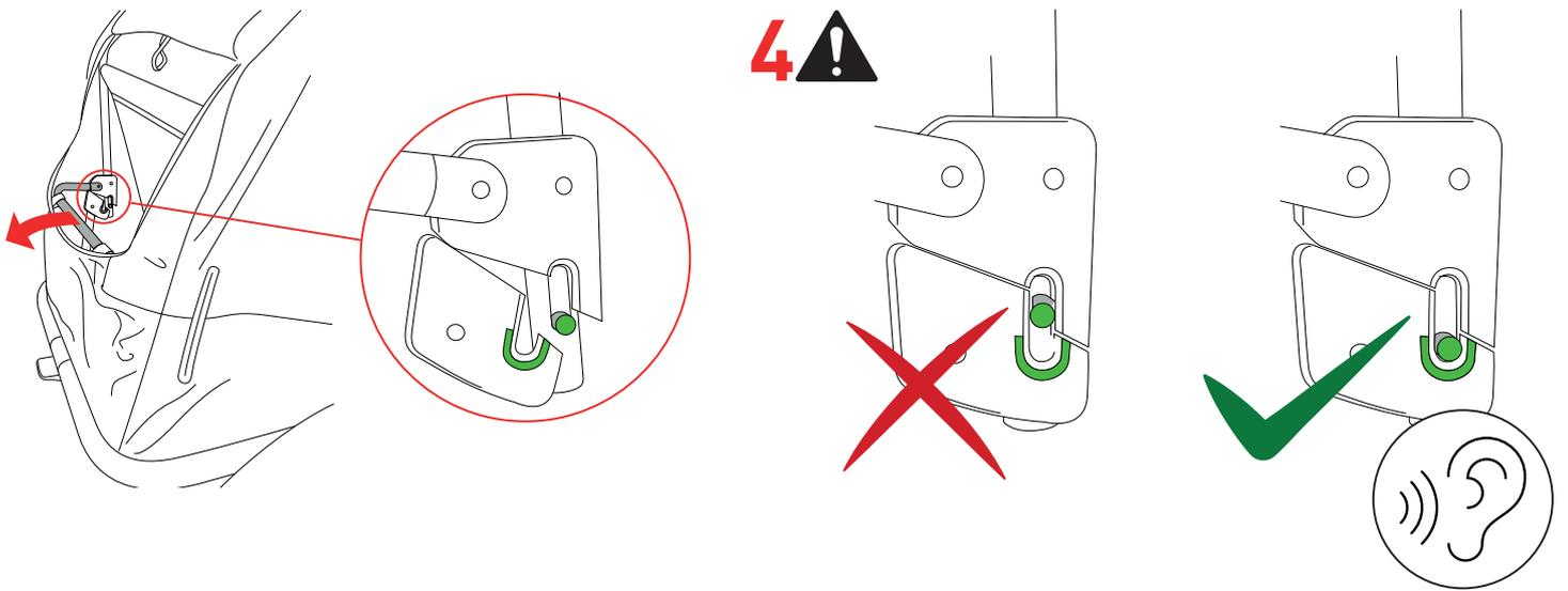
REIFENSCHUTZMONTAGE UND DEMONTAGE / WHEELGUARD ASSEMBLY AND DISASSEMBLY
