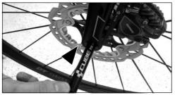
2. Secure the thru axle hand-tight with an Allen key.
