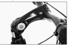
Many bikes are fitted with an adjustable stem, the height and angle of which can be adjusted. Only have the adjustment made in a specialist workshop!
