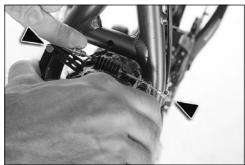
• Insert the cable in the yoke.
