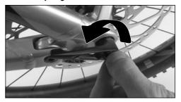
4. Once you have tightened the axle enough, position the lever so that it points towards the front-end of the bike and slide the lever onto the axle. Now turn the fixing screw 180° clockwise to secure the lever against working itself loose.
