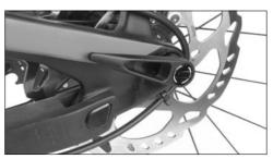
The lever can now be pulled slightly away from the axle and turned into any position you choose. To retighten the axle, reposition the lever on the axle in a comfortable position and tighten the torque again.
