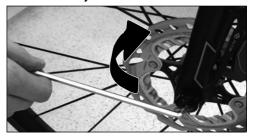
Then adjust the torque to the manufacturer-specified value using a torque wrench, but never exceeding 16 Nm.
