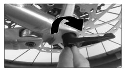
5. To release the axle, turn the lever anticlockwise. If you cannot apply enough force to the lever in the current position, follow steps 1 to 4 in reverse. Then you can adjust the position of the lever to make it easier to loosen.
