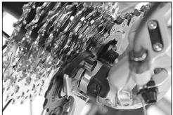
• Carefully lower the rear of the bike until the axle is at the dropout stop on the right and left sides.
