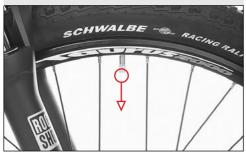
The valves must point directly towards the centre axis of the road wheel.
