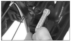
Swivel the locking lever so that the brake is fixed in place again.
