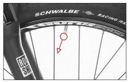
The valve does <u>not</u> point to the traversing wheel centre
