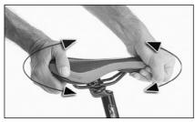
Try to move the saddle in its clamp with alternate up and down movements. It should not be possible to move the saddle.
