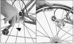
• Carefully lower the rear of the bike until the axle is at the dropout stop on the right and left sides.
