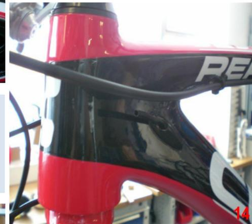
The final work step is to slide the the cable housing on the cable of rear derailleur. Now your bike is finally assembled and in a roadworthy condition. The importants utensil is definitely the assembling assistance (liner) which simplifies the replacing of the cables. **You can order a linerset at your distributor.**
