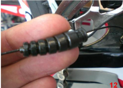
Up next you can drag the liner out of the hole in the bottom bracket housing, which is laid round this housing. Now you pull the long liner (1m) over the old shifting cable. (13)
