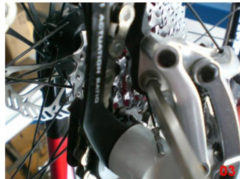
At first you loosen the shift cable at the rear derailleur and the screw of the cable stroke at the bottom of the chainstay. (2-3)
