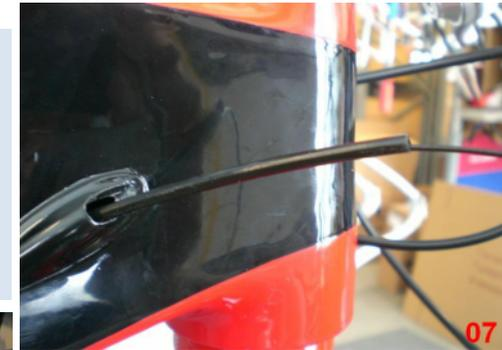
After you insert the new shifting cable into the liner you pull the liner out of the downtube. (8-9)
