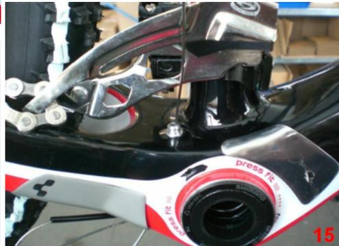
Finally you pin the cable of the front derailleur through the little hole of the bottom bracket housing. After that you put on the sealing and fix the cable with the screw of the front derailleur correctly.
