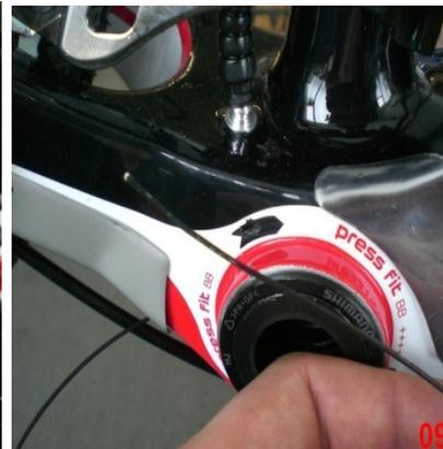
If the shifting cable should be changed too, it's the point in time. In case of only changing the rear shifting cable, you just have to disassembly the cable housing and the cable stroke.
