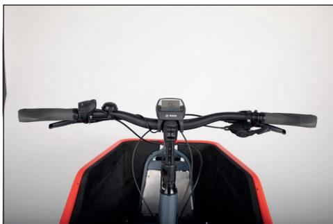
**Bild:** Handlebars with handlebar stem (including Speedlifter)
