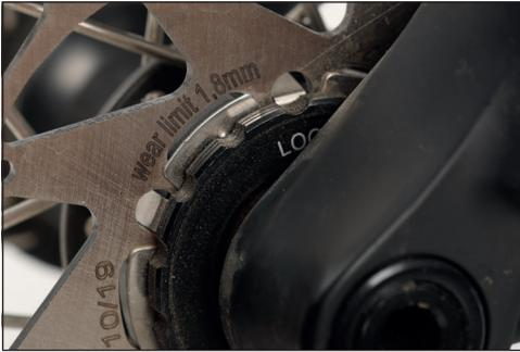
**Bild:** Information on the minimum thickness on the brake disc (1.8 mm)
