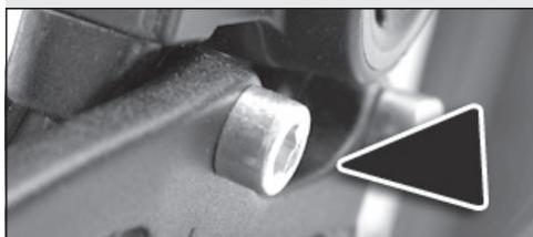
**Screw connection, not correct** A loose screw is often indicated by a protruding screw head.
