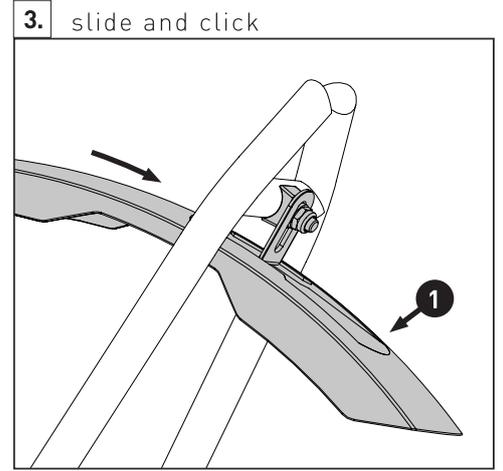
**MONTAGE MIT CUBE SIC ADAPTER HINTEN / assembly with CUBE SIC adapter rear**
