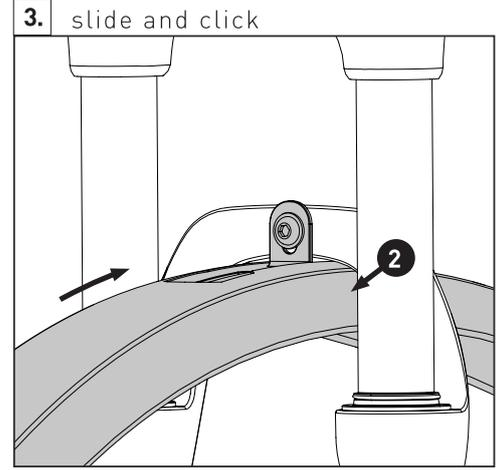
**MONTAGE AN SITZSTREBENBRÜCKE HINTEN / assembly on seat stay bridge rear**
